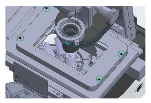
Install the base of the Nikon LSC using  $4 \times QG-0543-SK-100002$  (M3 x 14 Cap Head Screws).
