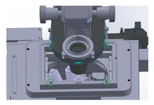
**Caution:** Use of incorrect length screws to install the Nikon LSC on to the piezo laser safety adapter could result in incorrect operation or damage to the piezo stage.
