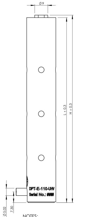
legacy model equivilent size MODEL Н L DPT-C-S-UVAC DPT-E-020-UHV 40.5 44.2 DPT-E-050-UHV 75 76.7 DPT-C-M-UVAC DPT-E-110-UHV 126.1 127.8 DPT-C-L-UVAC
